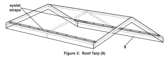
3. Place the Roof Tarp (9) over the top of the roof assembly with its eyelet straps facing down, on the inside.
